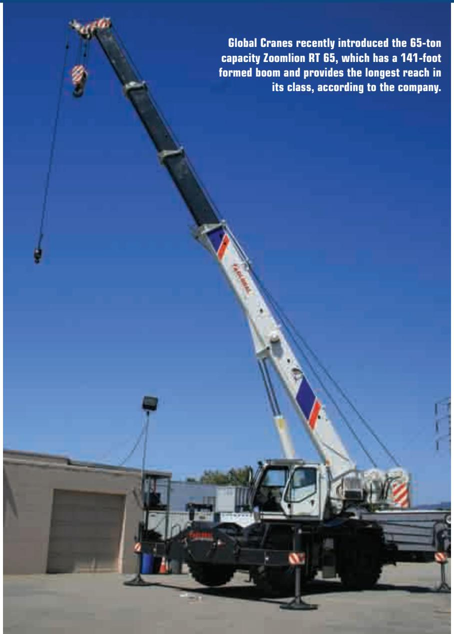
Global Cranes recently introduced the 65-ton capacity Zoomlion RT 65, which has a 141-foot formed boom and provides the longest reach in its class, according to the company.
